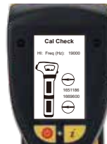
The self-test feature checks that the receiver is operating correctly, and the calibration has not drifted.
