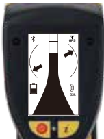
The standard locate screen shows the peak response indicator and line direction compass.
