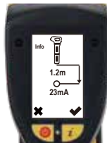
Press the z button for a depth reading with current measurement and logging options.
