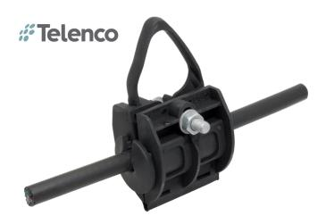
The Telenco® DS suspension clamps are designed to provide a mobile suspension for 5 to 17mm aerial round ADSS cables. These clamps are to install on intermediate poles used for the roll-out of access networks where spans do not exceed 70m.
