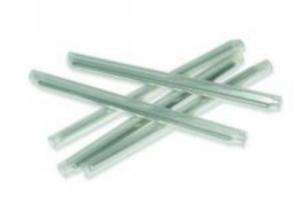
45mm Splice Protection Sleeves are high-quality heatshrinkable sleeves designed to protect fibre optic splices. Featuring a durable transparent outer tube and a reinforcing steel or ceramic rod, these 45mm sleeves provide robust protection for spliced fibres, ensuring the splice is shielded from environmental factors like moisture, dust, and temperature changes
