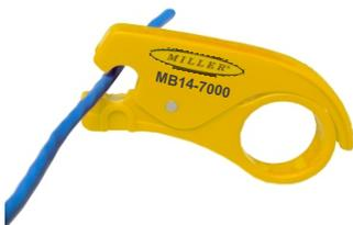
1. Squeeze handles to open the tool and locate cable in the jaws.
