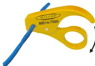
2. Rotate the tool one or two turns to score the jacket.
