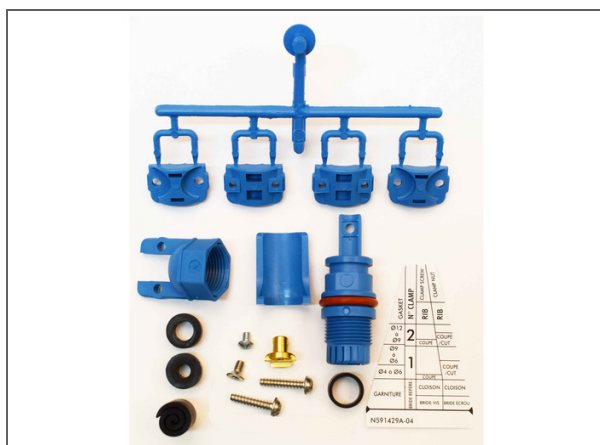
ECAM External Cable Assembly Module for BPEO, BPEO ECAM S12 ROUND CSM Single-Entry Cable Sealing seals and anchors round shape cables with outside diameter from 4 to 12 mm with a Central Strength Members
